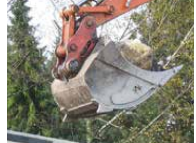
Standard tooth system is Esco Super V, other systems on customer request
